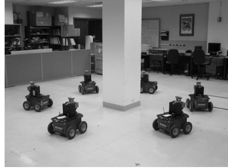
Fig. 2. Six Pioneer robots in defensive formation around support column are about to receive request to change swarm radius.
