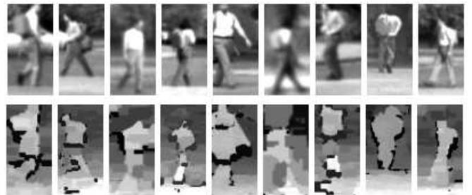
Fig. 6. Sample mid-range inputs showing image and disparity maps.
